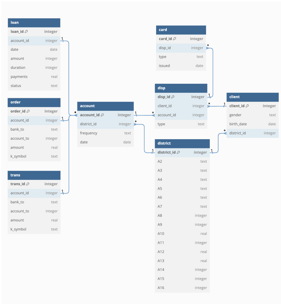
Figure 4: Database schema of the database in the financial domain of BIRD-Bench.
